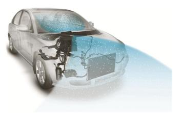
Optional Multi filter<sup>1</sup>- Cars equipped with the Interior Air Quality System (IAQS) are equipped with a multi-filter. The multi-filter is electrostatically charged and impregnated with active carbon. The carbon absorbs harmful substances, such as unhealthy air pollutants in exhaust fumes. It also does an excellent job of absorbing unpleasant gases and odors.
